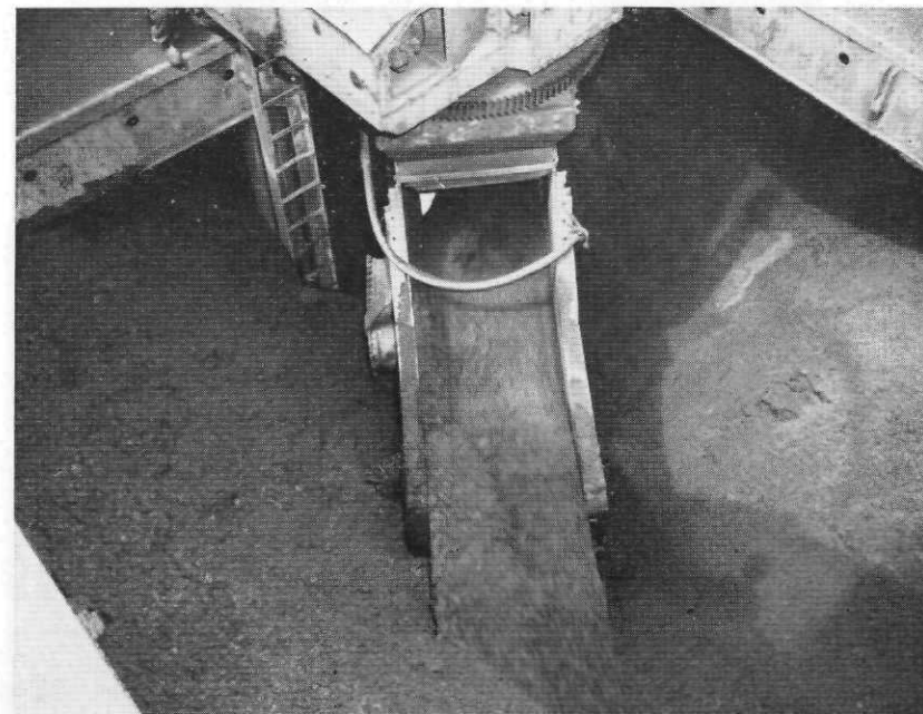
The trimmer can be turned in all directions to load all parts of the hold without necessity for manual trimming.
